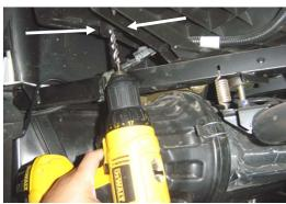
After mounting the pod, drill up through the hole in the bottom of the bed using the 1/4" drill bit , this is where your speaker wire will run into the pod
