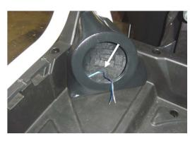
Run the speaker wire into the pod using the hole in the bottom
