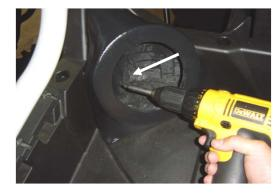
Align the Kick Panel in the corner of the bed and screw into the plastic using the 3 provided screws
